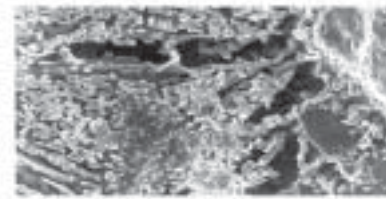
High concentration of acid produces fines in pores
